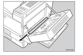
Open the right cover by pushing the catch upwards.
