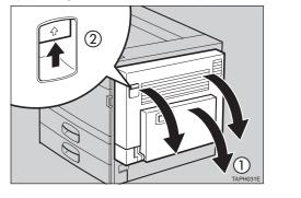
Remove the packing material as shown in the illustration.
