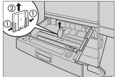
Align all four sides of the paper stack and load it into the tray.
